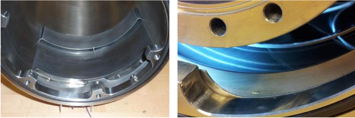
Figure 5.8: The stainless steel support saddle is supporting the big quartz tube. Right: design of the saddle and supposed position within the vacuum chamber. Left: the inner electrode of the big quartz tube has a direct line-of-sight onto the grounded saddle.
