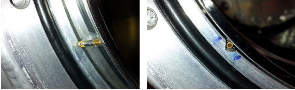
Figure 5.5: In order to be able to insert the medium quartz tube into the system a groove had to be filed into the custom made extension chamber. In the left figure the ground connector of the outer electrode does not fit into the extension. The figure to the right shows the groove which was filed in allowing to insert the quartz tube with its ground connector.
