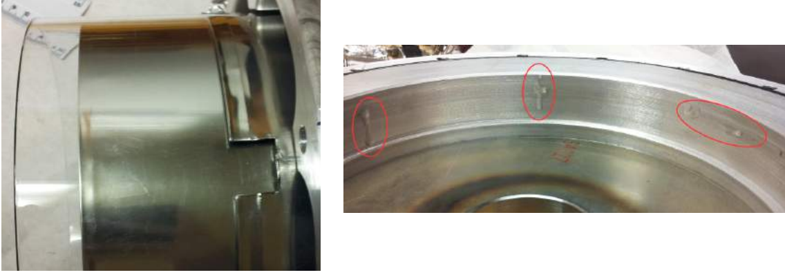
Figure 5.7: The left figure shows that notches have been cut out of the outer electrode foil on the medium quartz tube. The notches are located in a high field region according to [84]. The right figure shows where the sealant penetrated into the vacuum chamber can be seen.
