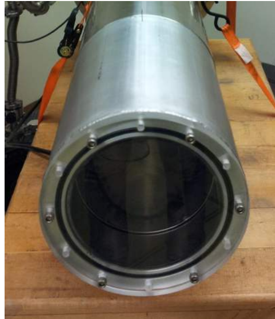
Figure 5.4: To the right the custom made blanking plate with a HV feedthrough and a pump port is shown. The acrylic observation window attached to a custom made extension is shown on the right side.
