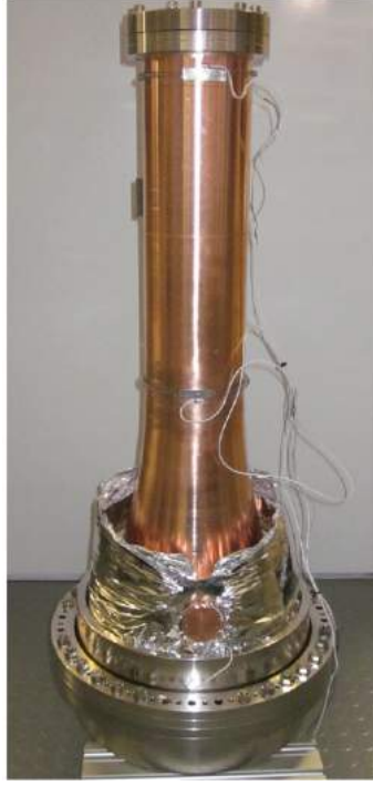
Figure 4.2: Post-Acceleration-Electrode of the FPD system. Picture adapted from[63].
