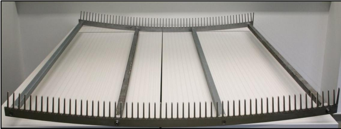
Figure 4.3: **A photograph of a double-layer wire electrode module** from the cylindrical part of the main spectrometer. The wires are stretched between the comb-like structures. From [26].
