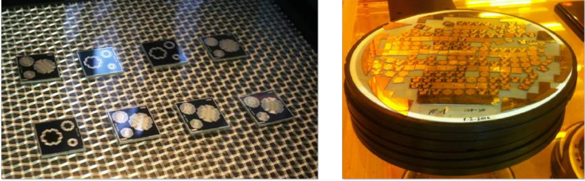
Figure 3.4: Pictures of HLL sensors. Three different detectors with seven pixels each are placed on one squared chip. The sensors all come from the same monolithic silicon wafer.
