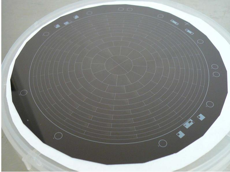
**Figure 3.7.:** The detector wafer. For spacial resolution it is segmented into 148 equal area pixels arranged in 12 concentric rings with 12 pixels each plus an additional four-pixel bulls eye in the center. Figure adapted from [Wal13].
