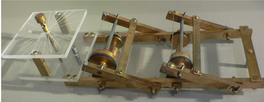
Figure A.1.: The FERMIAC, invented by E. Fermi. The FERMIAC is an analog computer using Monte Carlo method to study slow neutrino transport. It is one of the first applications of Monte Carlo methods for modern physics. (Picture from [Com17])
