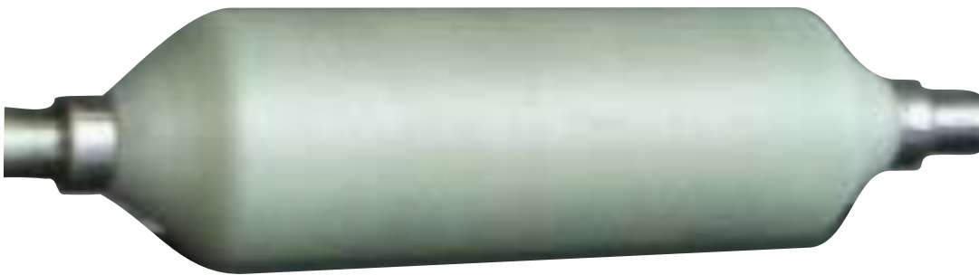
Figure 3.14: The GFP insulator. The insulators of the Babcock Noell GmbH. The triple junction is recessed to prevent voltage breakdowns.
