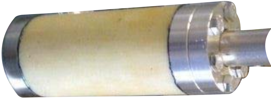
Figure 3.11: The GFP insulator. One glass fibre-reinforced plastic insulator is shown. The flanges are made for indium seals.
