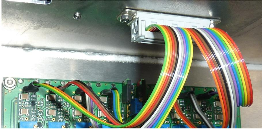
Figure 5.12.: **Picture of the New Signal Feedthrough for the Veto** in the lower part of the veto box. A ground connection for each MPPC was added replacing a single ground connection to the aluminum bar which houses the MPPCs.
