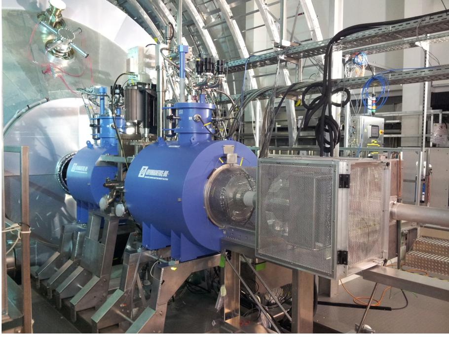
Figure 5.1.: **The FPD System Installed at KIT** prior to its connection to the main spectrometer. The Data Acquisition Crate and the High Voltage Crate are out of the picture on the right hand side.
