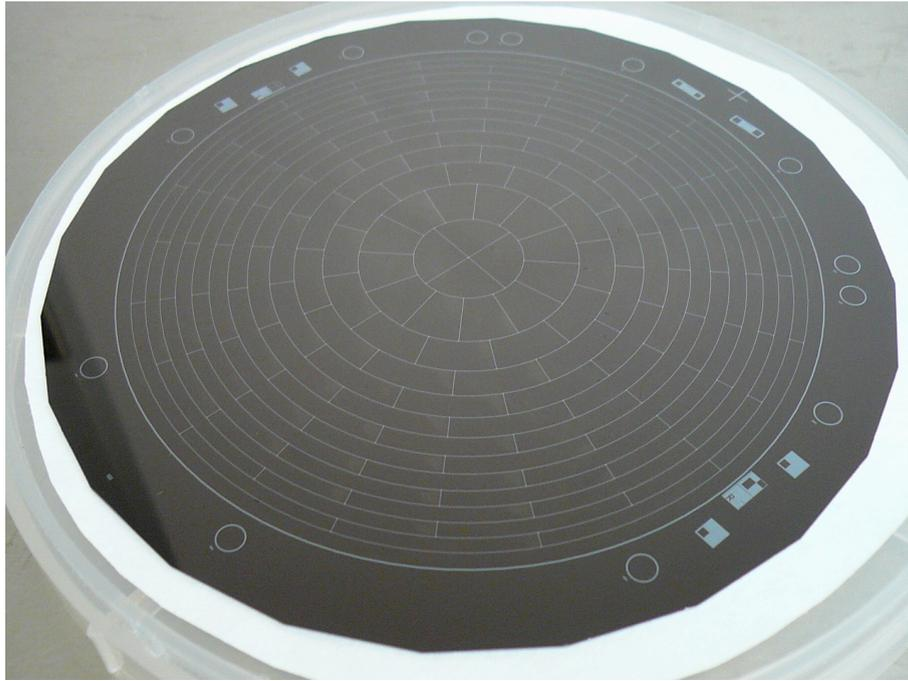
Figure 5.5.: **Picture of the Detector Wafer's Segmented Backside.** The 148 pixels arranged in twelve concentric rings plus four "bulls-eye" pixels are shown in addition to the guard and bias ring at the insensitive outer regimes of the wafer (From [1]).
