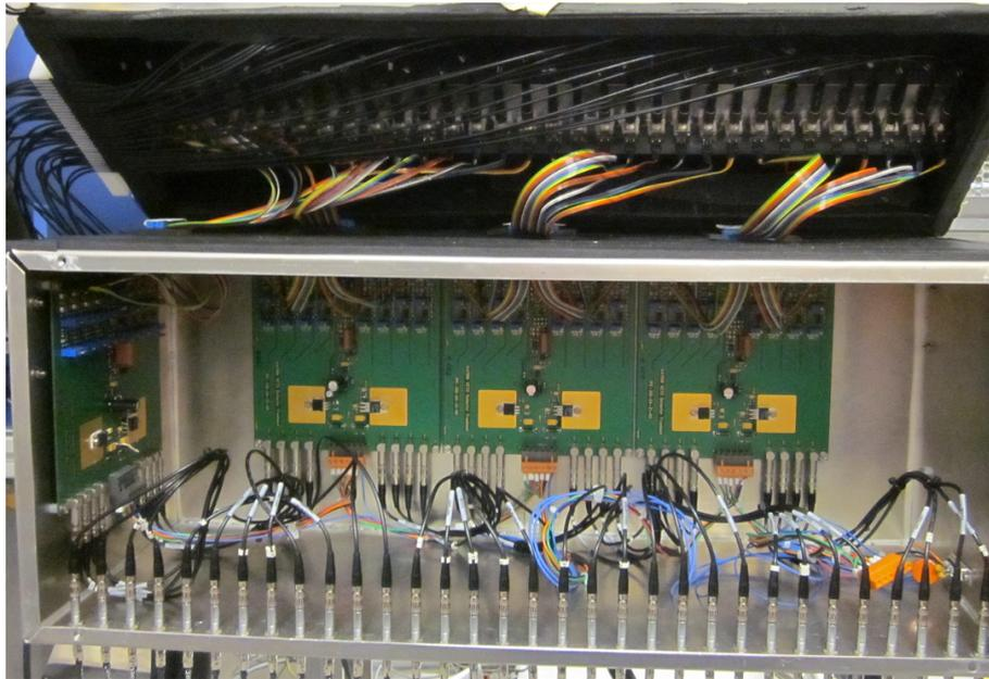
Figure 5.11.: **Picture of the Veto Readout Electronics Box** with the upper part lifted up to show the aluminum bar that supports the MPPCs which in this picture are connected to the veto panels by optical fibers. The four amplifier boards are located in the lower part of the box.
