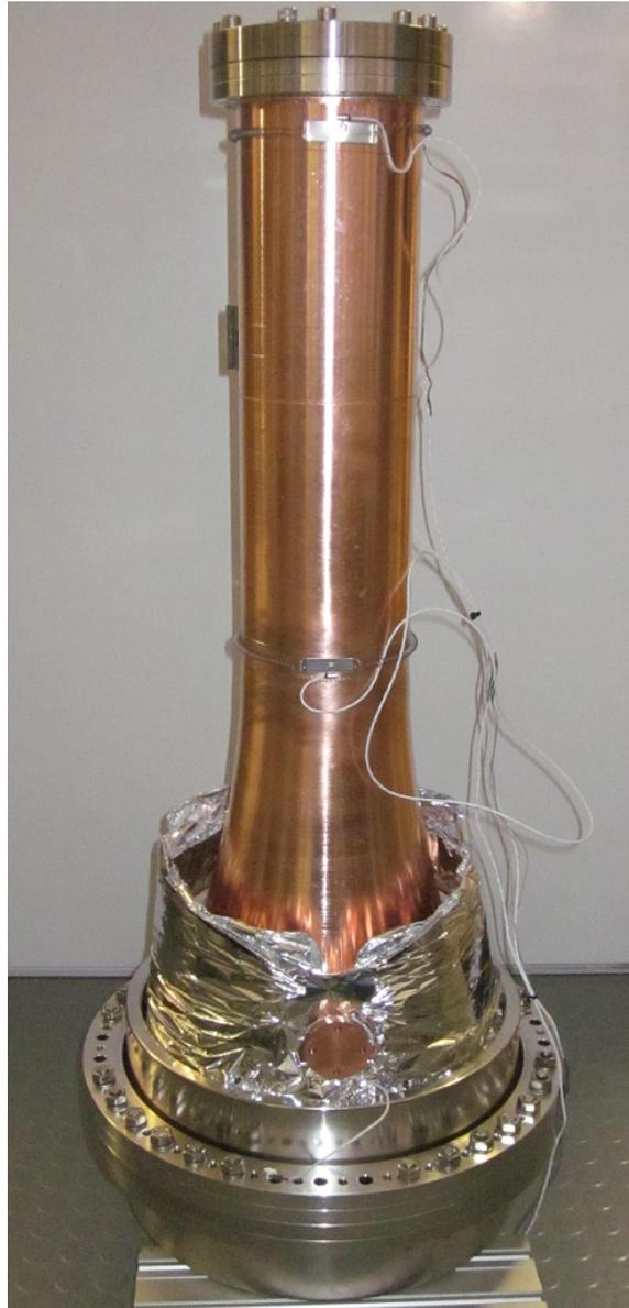
Figure 5.4.: **Picture of the New, Mechanically more Robust Post-Acceleration Electrode.**
