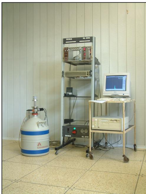
**Fig. 6.** The Canberra Si(Li)  $\gamma$ -spectrometry apparatus.
