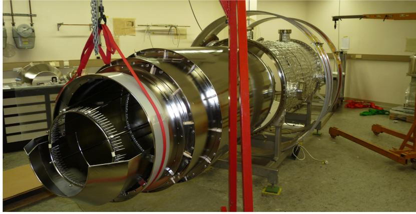
**Figure 3.2.:** Cylinder- and wire electrode are seen in a configuration where the spectrometer was disassembled for the transport. In the background the stainless steel tank and three air coils are visible.
