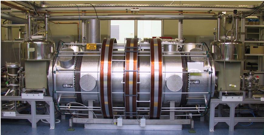
**Figure 3.1.:** Monitor spectrometer, consisting of the thermally insulated tank, the two superconducting solenoids and the air coils.
