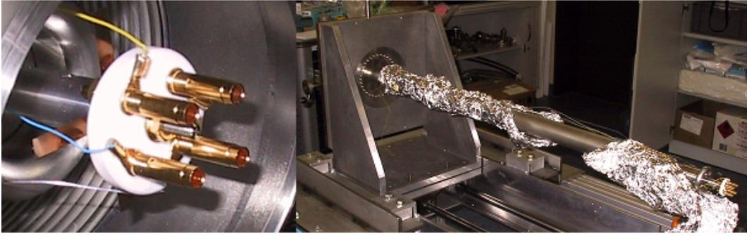
**Figure 3.9.: Sourceholder** The left side shows the sourceholder. The sources sit on banana plugs, which can be plugged into the respective banana socket. Behind the ceramic plate the centering cross made out of spring bronze can be seen. The cross is electrically isolated so that it can be detected when it touches the wall. Visible are also the cables which allow to set the potential on each source individually. On the right side the tube on which the sourceholder is placed can be seen.
