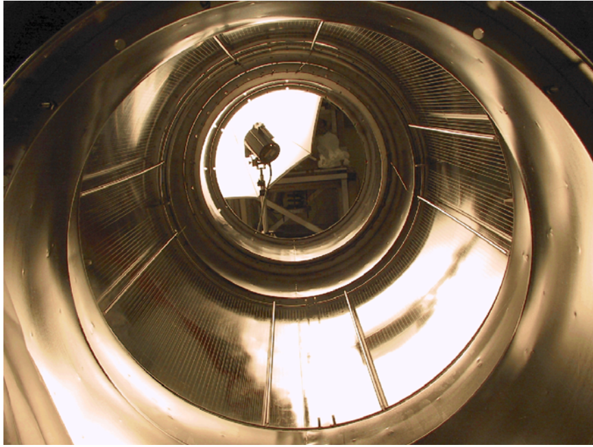
Figure 11: The upgraded electrode system of the Mainz spectrometer with its new central dipole electrode. The wire-based electrode was built in April/May 2002.
