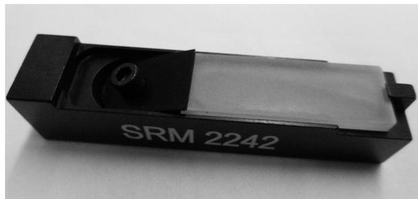
**Figure 4.4:** The luminescence standard SRM 2242. The actual glass slide is delivered in an optical mount, as can be seen here. For the use in the LARA setup, this mount is replaced by a custom one.
