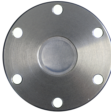
Figure 4.6: Materion IF-1 beryllium window in DN40 CF flange. The picture shows the beryllium window before it was sputter-coated with gold. The coated window, mounted inside the recipient is shown in figure 4.7.
